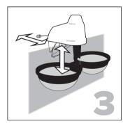
Push the white leveling device in from the back of Fry Factory along the top of the metal clip. Pull white leveling device out, to lower the nets into the water. Push the white leveling device in, to lift the nets out of the water.
